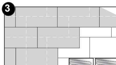
This method of installation will provide a stable surface for the floor finish to rest on and avoid any joints showing through the final floor finish.
